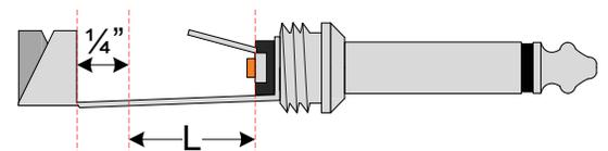
3. Remove a length (about equal to "L") of the cable's outer jacket from the cable end exposing the copper shielding beneath it. **Be careful not to accidentally cut through any of the shielding.**
