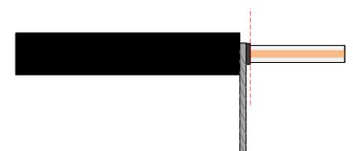
6. Remove  $\frac{1}{4}$ " of the center insulation from the cable end. *Be very careful not to cut off any of the strands from the center conductor.* Twist and tin the exposed center conductor strands together.
