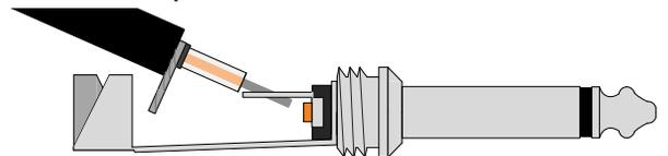
9. Connect the shield conductor to the sleeve terminal:
