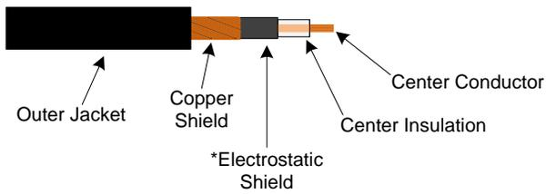
\*The electrostatic shield acts as a semi-conducting barrier between the copper shield and the center insulation to discharge static electrical charges generated when the copper shield rubs against the insulation. This eliminates crackling noises that could otherwise be heard when the cable is moved.
