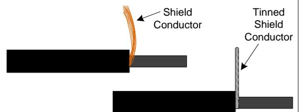
5. Remove the electrostatic shield from the cable end starting as far back as you can above the tinned shield conductor. **The electrostatic shield is very thin, so be careful not to cut through the insulation beneath it.**
