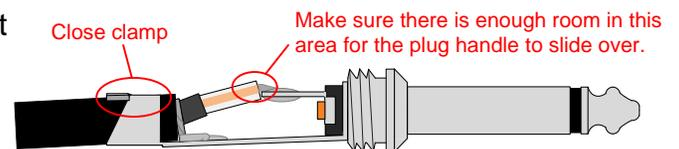
11. Push the plug handle and insulator over the connections. (The insulator helps ensure the tip terminal will be insulated from the shielded handle). Screw the handle onto the  $\frac{1}{4}$ " plug's threading and that cable end is done.
