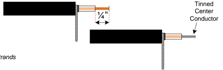
7. Cut the shield conductor to a length between  $\frac{1}{4}$ " and  $\frac{1}{2}$ ", according to your preference.
