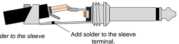
10. Close the cable clamp tightly around the outer jacket of the cable.
