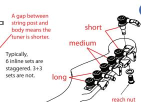
Insert the tuner shafts through the plate and headstock holes.
