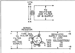
Typical circuit to provide regulated supply voltage of approximately 75, 105, or 150 volts to load. Removal of tube from socket removes voltage from load.
